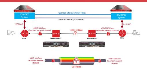
Ciena and ID Quantique demonstrate how 400Gbps MACsec quantum-secured channels can enable network operators to detect and defend against eavesdroppers across metro applications. The demo features Ciena's 8140 Coherent Aggregation Router leveraging open APIs to communicate with ID Quantique's Quantum Key Distribution (QKD) Cerberis XGR platform.
